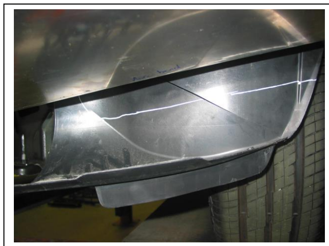
Figure 15: Mark and trim guard liner to fit rear of underbelly guard.
